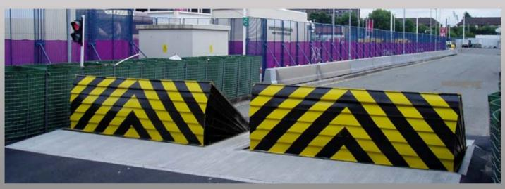
Successfully impact tested to the latest PAS 68:2010 specification stopping a 7500kg vehicle travelling at 50mph (80kph) which equates to 1852kJ. Maximum width 4000mm. Surface Mounted.
