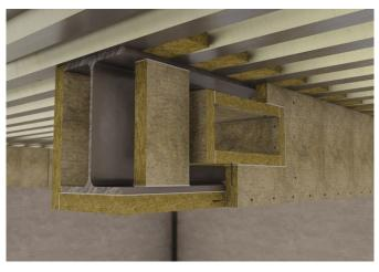
Figure 12 - Beam with square or rectangular holes (boxed and profiled protection - glued and pinned joints)
