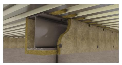
Figure 9 - Stud welded pins and board-to-board glued joints (Up to 4 hours fire protection)
