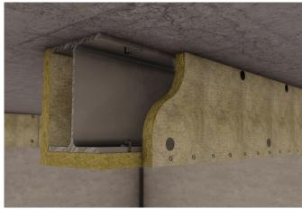
Figure 3 - Clip and stud welded pin dry joint system (Up to 2 hours fire protection)
