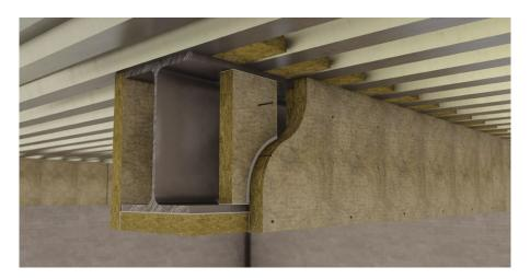
Figure 8 - Glue-fixed noggins and board-to-board glued joints (Up to 4 hours fire protection)
