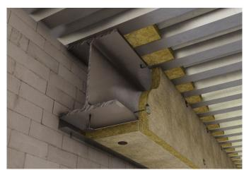
Figure 7- Two-sided protection with stud welded pins (Up to 2 hours fire protection)
