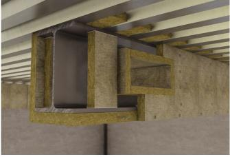
Figure 14 - Beam with square or rectangular holes (boxed protection - dry joints)
