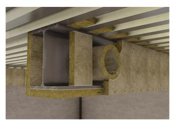
Figure 11 - Beam with circular holes (boxed and profiled protection - glued and pinned joints)
