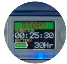
Colour coded display showing remaining battery life
