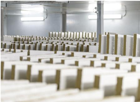
In turn this is melted in a furnace at a temperature in excess of 1500°C. As the molten liquid rock pours from the furnace, nature's process is recreated. Lava flow is directed into a chamber where it is spun and transformed into rock strands and stone wool, the core of our Stopseal Batt system. A FSi specially designed and tested coating is applied to this core at a predetermined thickness, protecting the core from fire, thus creating the Stopseal® Batt as seen today.
