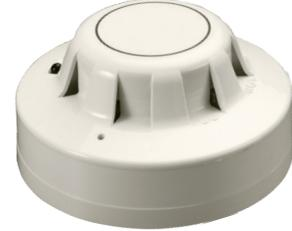
The Series 65A Ionisation Smoke Detector uses a low activity radioactive foil to detect fires by irradiating the air in the smoke chamber causing a current flow. If smoke enters the chamber, the current flow is reduced leading to an alarm.
