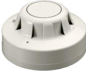
The Series 65A Photoelectric Smoke Detector incorporates a pulsing LED located within the housing of the detector. The detector has an indicator LED which is clear in a quiescent state but produces a red light when in alarm.
