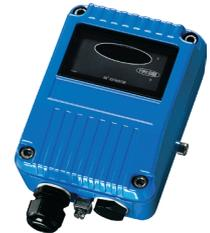
The Conventional I.S. IR<sup>3</sup> Flame Detector is designed for harsh environments in either indoor or outdoor applications. It is sensitive to low-frequency flickering IR radiation emitted from flames during combustion. The sensor operates even through a layer of oil, water vapour or ice. These detectors have been approved by BASEEFA to EN 50014, EN50020 and EN50284. The requirements of the ATEX Directive 2014/34/EU have also been met.
