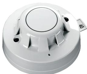
The Discovery Ionisation Smoke Detector uses a low activity radioactive foil to detect fires by irradiating the air in the smoke chambers and causing a current flow. If smoke enters the chamber, the current flow is reduced leading to an alarm.
