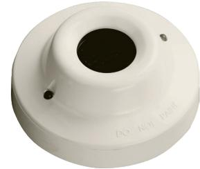
The Intelligent Base Mounted IR<sup>3</sup> Flame Detector is designed to protect all indoor areas, even in dirty or smoky conditions, where open flaming fires may be expected. The detector has three IR sensors that respond to different IR wavelengths in order to discriminate between flames and spurious sources of radiation.
