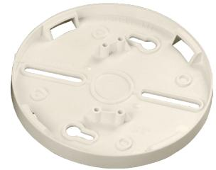
The Sounder Ceiling Plate allows surface-mounted cabling to be fitted to a loop-powered sounder base.
