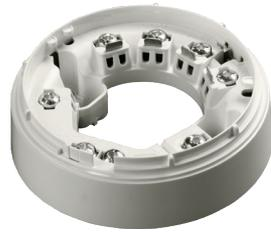
The Orbis Marine Relay Base incorporates a single-pole voltage-free changeover contact for switching ancillary equipment. When the detector changes to the alarm state, the relay is energised, causing the contact to change state. The contact will remain in this condition until the detector is reset.
