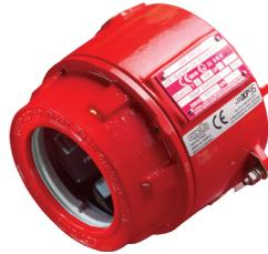
The Intelligent Flameproof IR<sup>3</sup> Flame Detector is designed for hazardous environments in either indoor or outdoor applications. It is sensitive to low-frequency, flickering infra-red radiation emitted by flames during combustion. These detectors are BASEEFA approved and meet the requirements of ATEX Directive 94/9/EC.
