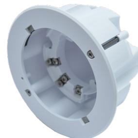
A polycarbonate mounting box for installing the Soteria Dimension detectors. This mounting box is installed into the ceiling void or pre-set in a solid ceiling. The loop is wired to this mounting box which contains the connectors for the Soteria Dimension detectors.
