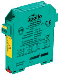
The DIN-Rail Mains Input/Output Unit provides a voltage-free, single pole changeover relay output and a monitored switch input. The unit supervises one or more normally-open switches connected to a single pair of cables.
