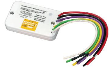
The XP95A Mini Priority Switch Monitor Module is designed to monitor the state of one or more single pole, voltage-free contacts and to report this status to Apollo-compatible analogue control equipment. It can also place a signal on this loop to provide early warning if a device such as a pull station is operated.
