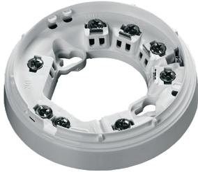
The TimeSaver<sup>®</sup> Relay Base incorporates a single-pole voltage-free changeover contact for switching external equipment. When the detector changes to the alarm state, the relay is energised, causing the contact to change state. The contact will remain in this condition until the detector is reset.
