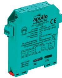
The DIN-Rail Zone Monitor with Isolator powers and controls a zone of up to 20 Apollo Series 65 or Orbis fire detectors in a Discovery or XP95 loop.
