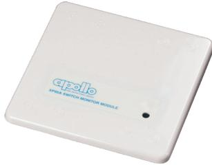
The XP95A Switch Monitor Module is designed to monitor the state of one or more single pole, voltage-free contacts and to report this status to Apollo-compatible analogue control equipment.
