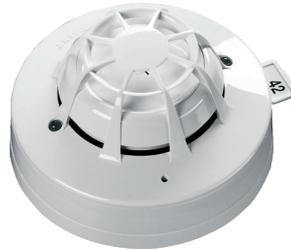
The Discovery Optical/Heat Multisensor Detector comprises optical smoke and thermistor temperature sensors which give both a combined signal as well as a separate heat signal for improved false alarm management.
