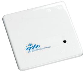
The XP95A 120V AC Input/Output module is a loop-powered device which incorporates a monitored input circuit for connection to dry contacts, in addition to a 120V AC 4A rated dry contact relay output. It is mounted in a plastic fascia plate for use with a 4 square or two-gang electrical back box.
