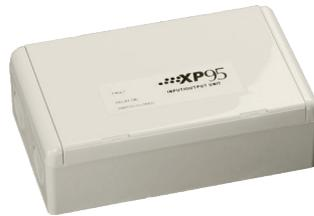
The Input/Output Unit provides a voltage-free and double pole changeover (DPCO) relay output, a single monitored switch input and an unmonitored, non-polarised opto-coupled input.
