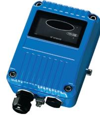
The IR<sup>3</sup> flame detector is designed for harsh environments in indoor applications. The detector has three sensors which respond to different IR wavelengths to discriminate between flames and spurious sources of radiation.
