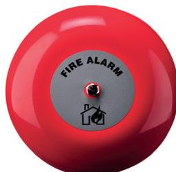
The conventional 6" Fire Bell is a motorised bell designed for fire alarm applications. Its low current consumption and universally recognisable alarm sound makes it an ideal choice for many alarm systems. Designed for ease of installation, it features a robust steel gong.
