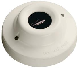
The Intelligent Base Mounted UV Flame Detector is designed to protect enclosed indoor areas where open fires may be expected. The detector has a fast-acting response to flames up to 25m away and is equipped with a single UV sensor with a narrow spectral response in order to discriminate between flames and most spurious sources of radiation.
