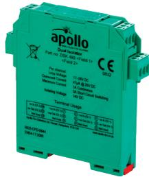
The DIN-Rail Dual Isolator provides two independent isolators which sense and isolate short-circuits on Discovery or XP95 loops and spurs.
