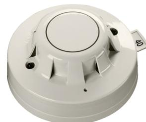
The Discovery UL Ionisation Detector uses a low activity radioactive foil to detect fires by irradiating the air in the smoke chambers and causing a current flow. If smoke enters the chamber, the current flow is reduced leading to an alarm.
