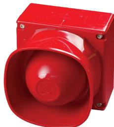
The Multi-Tone Weatherproof Open-Area Sounder is designed for use in open areas and can be connected to an XP95/Discovery system. The sounder comprises a backbox and sounder unit supplied together.
