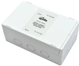
The Intelligent Twin Switch Monitor provides the function of two Switch Monitor units within one enclosure. The two units are electrically independent of each other. There is a DIL-switch on each unit to set the address.
