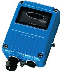
The IR<sup>2</sup> flame detector is designed for harsh environments in indoor applications. The detector has two sensors which respond to different IR wavelengths to discriminate between flames and spurious sources of radiation.
