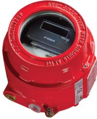
The Intelligent Flameproof IR<sup>2</sup> Flame Detector is designed for hazardous environments in indoor applications. The detector has two sensors which respond to different IR wavelengths to distinguish between flames and spurious sources of radiation. These detectors are BASEEFA approved and meet the requirements of ATEX Directive 94/9/EC.
