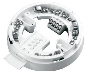
The Intelligent Heater Base is designed to be used in cold climates where environmental conditions could result in either icing or condensation affecting the operation of detectors. It is recommended that the heater base be used in conjunction with either a Waterproof Base Cover or Deckhead Mounting Box to minimise moisture ingress.
