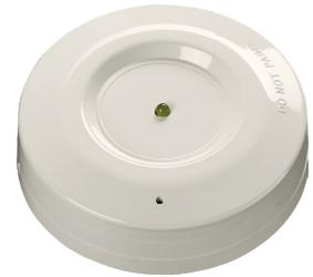
The Discovery Marine Isolator is placed at intervals on the loop and ensures that, in the case of a short-circuit, only the section between the isolators will be affected. When the short-circuit is removed, the isolators automatically restore power and data to the isolated section.
