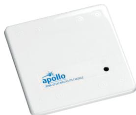
The XP95A 120V AC Input/Output module is a loop-powered device which incorporates a monitored input circuit for connection to dry contacts, as well as a 120V AC 4A rated dry contact relay output. It is mounted in a plastic facia plate for use with a 40 square or two-gang electrical back box.
