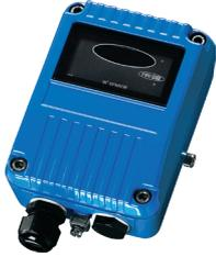
The Conventional I.S. IR<sup>3</sup> Flame Detector is designed for harsh environments in either indoor or outdoor applications. It is sensitive to low-frequency flickering IR radiation emitted from flames during combustion. The sensor operates even through a layer of oil, water vapour or ice. These detectors have been approved by BASEEFA to EN 50014, EN50020 and EN50284. The requirements of the ATEX Directive 2014/34/EU have also been met.
