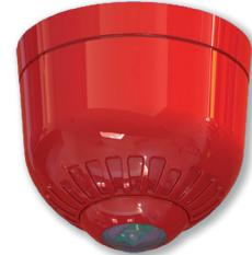
Conventional ceiling mounted Visual Alarm Devices are available with a white and red flash colour. The white flash variant has an EN 54-23 approved coverage pattern of C-3-15, whereas the red flash variant has a coverage pattern of C-3-8.9.
