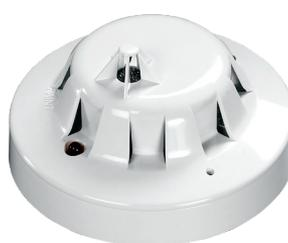
The Discovery CO/Heat Multisensor Detector is good at detecting deep-seated smouldering fires which produce a lot of CO as well as flaming fires. They are ideal for use in hotel bedrooms where steam may be present, dusty environments or even locations where simulated smoke may be present.
