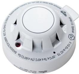
The XP95 I.S. Optical Smoke Detector works using the light scatter principle and is ideal for applications where slow-burning or smouldering fires are likely.
