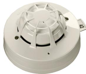
The Discovery Marine Optical/Heat Multisensor Detector comprises optical smoke and thermistor temperature sensors which give both a combined signal as well as a separate heat signal for improved false alarm management.
