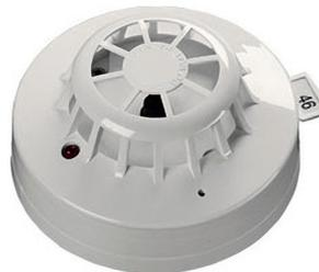
The XP95A Heat Detector monitors temperature by using a single thermistor which provides a voltage output proportional to the external air temperature. It is classified as an ordinary detector by UL.
