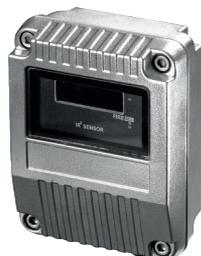
The Stainless Steel Intelligent IR<sup>3</sup> Flame Detector combines high performance with added protection against the effects of salt corrosion, making it ideal for most marine applications. The protection from salt corrosion, is provided by a tough, heavy-duty housing made from stainless steel material. It can rapidly detect all types of flames, including hydrogen, which is invisible to the human eye.
