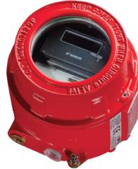
The Flameproof UV/IR<sup>2</sup> Flame Detector is designed for hazardous environments in either indoor or outdoor applications where open fires may be expected. False alarms from flickering sunlight, arc welding or lightning are avoided by the combination of UV and dual IR signal processing techniques. It detects almost all flames, including those invisible to the naked eye, e.g. hydrogen fires. Certified by ISSOP for compliance with standards EN 50014, EN 50018 and EN 50281.
