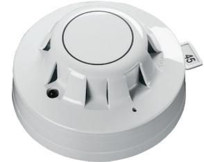
The XP95 Ionisation Smoke Detector uses a low activity radioactive foil to detect fires by irradiating the air in the smoke chambers and causing a current flow. If smoke enters the chamber, the current flow is reduced leading to an alarm.
