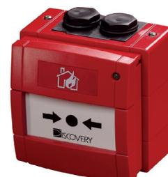
The Discovery Marine Waterproof Manual Call Point has been approved for use in outdoor marine applications. A seven-segment DIL switch enables addressing of each call point at commissioning stage. When operated, the manual call point interrupts the polling cycle for a fast response. Bi-coloured LEDs indicate isolate and normal conditions.
