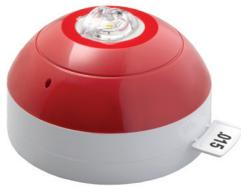
The Loop Powered VAD is designed for indoor use. The Wall VAD is specifically designed for use on the wall. The EN 54-23 coverage class for this device is W-2.5-7. These devices are to supplement sounders in areas which carry the risk that sounders will not be heard.
