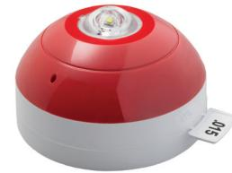
The Loop Powered VAD is designed for indoor use. The Ceiling VAD is specifically designed for use on a ceiling and comes in two different coverage classes. The two EN 54-23 coverage classes are C-3-8.5 and C-3 15. These devices are to supplement sounders in areas which carry the risk that sounders will not be heard.
