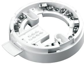
The Intelligent Deep Base is a mounting base for Discovery products which has an increased depth allowing for cables to be inserted from the side.
