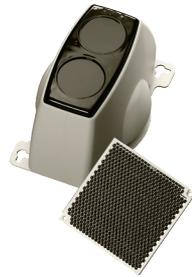
The Intelligent Reflective Beam Detector differs from a traditional beam detector in that it is a single unit which houses a transmitter, a receiver and the control electronics. The beam detector is available in two versions: a single reflector model for distances of 5-50m and a more powerful four-reflector unit for distances of 50-100m.
