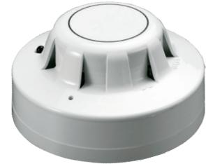
The Series 65 Ionisation Smoke Detector uses a low activity radioactive foil to detect fires by irradiating the air in the smoke chamber and causing a current flow. If smoke enters the chamber, the current flow is reduced leading to an alarm.
