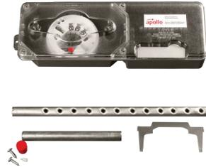
The Conventional Duct Smoke Detector provides early detection of smoke in the air moving through heating and ventilation (HVAC) ducts in commercial and industrial premises. Its purpose is to prevent the re-circulation of smoke from an area on fire to areas unaffected by the fire when used with a Series 65 or Orbis detector. It provides a volt-free changeover relay rated at 30V, 1A.
