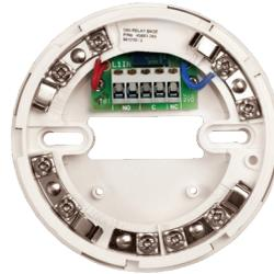
The Standard Series 65A Relay Base provides one set of volt-free, changeover (form C) contacts that change state when the detector signals an alarm.
