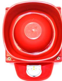
The Conventional Open-Area Wall Sounder VAD is used to provide audible and visual warning of a fire. Combining an EN 54-3 compliant sounder with an EN 54-23 compliant VAD enables this device to be used in areas that require the use of both an audible and a visual alarm.
