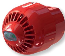
Conventional wall mounted Sounder Visual Alarm Devices are available with a white and red flash colour. The white flash variant has an EN 54-23 approved coverage pattern of W-3.1-11.3, whereas the red flash variant has a coverage pattern of W-2.4-7.5. The sounder has an SPL of up to 97dB.
