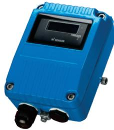
The Intelligent IR<sup>3</sup> Flame Detector is designed for harsh environments in either indoor or outdoor applications. It is sensitive to low-frequency, flickering infra-red radiation emitted by flames during combustion.
