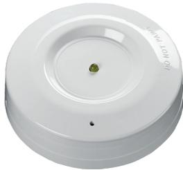
The XP95A Isolator is placed at intervals on the loop and ensures that, in the case of a short-circuit, only the section between the isolators will be affected. When the short-circuit is removed, the isolators automatically restore power and data to the isolated section.
