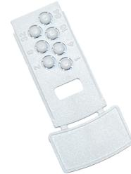
XPERT 7 Cards are supplied with all XPERT 7 Mounting Bases. Using a coding guide pips are removed to set the address of the inserted detector.
