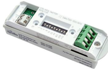
The Intelligent DIN-Rail Switch Monitor is designed to monitor the state of one or more single pole, volt-free contacts connected on a single pair of cables to report the status. It has a selectable status reporting delay making it suitable for monitoring flow switches.
